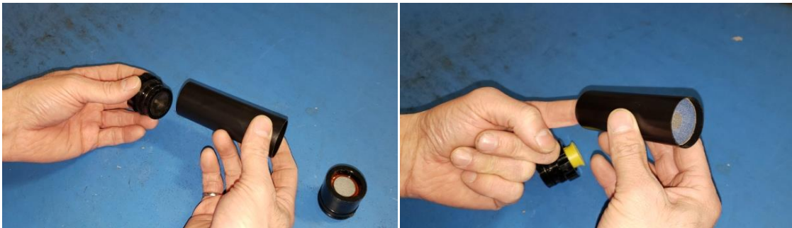
Figure 3: Removal of nozzle to extract or modify propellant grain.
