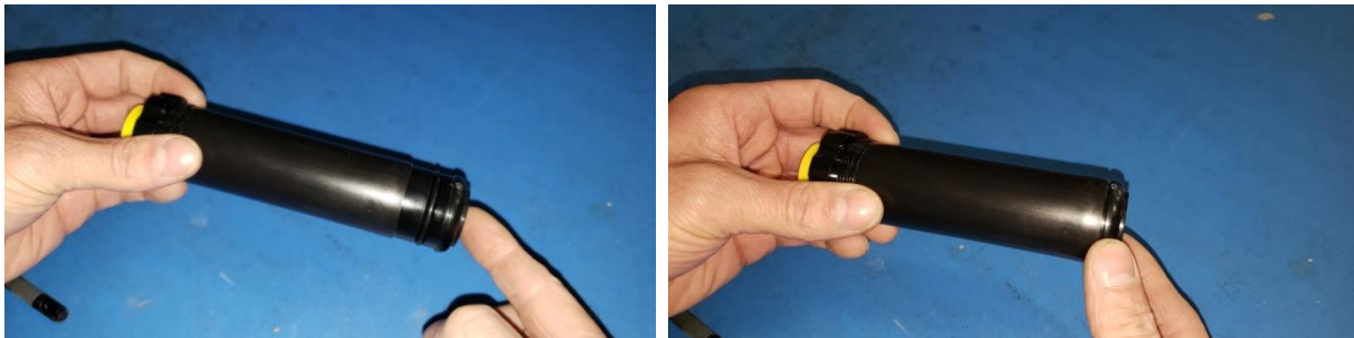
Figure 14: Re-assembly of forward closure , make sure the o ring is engaged into the liner.
