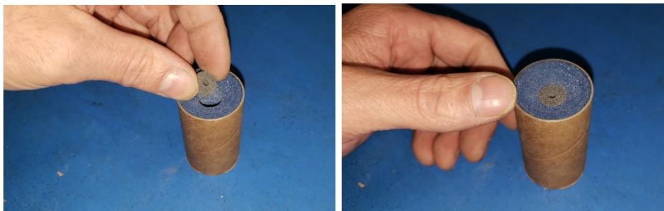
Figure 12: Pellet installation procedure, press into place with light pressure
