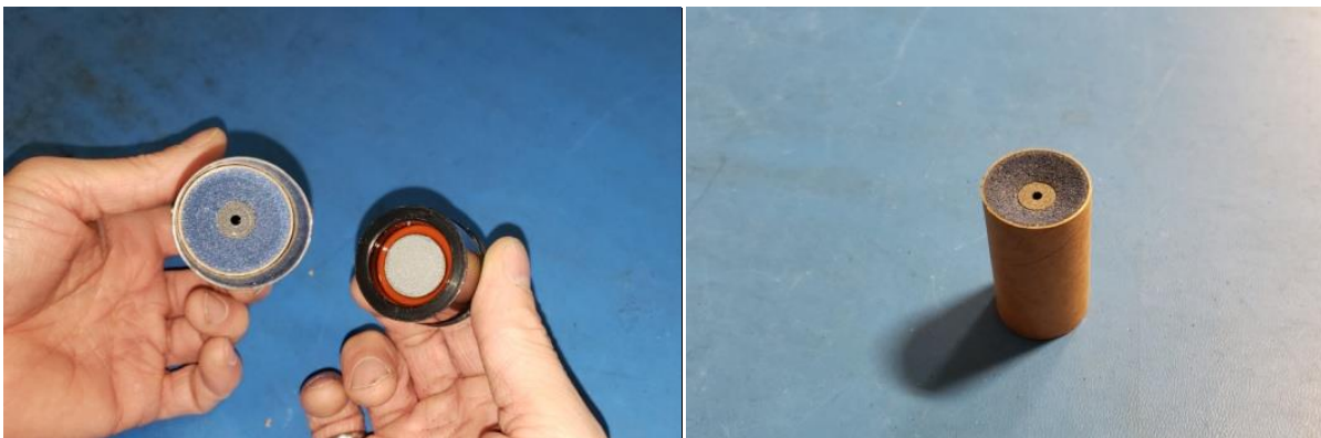
Figure 4: Grain with pellet assembly in forward section (i.e. bevel).
