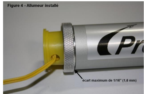
Figure 4 - Allumeur installé
